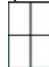
Fig 12c The lattice structure form for rectangles ,no loss in area , has large areas, use large amount of material. rectangular Perimeter =19,7cm
