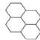
Fig 12a The lattice structure form for hexagonal, has minimum area, minimum material , no loss in area .Hexagonal perimeter=18cm.
